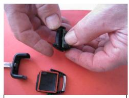
3. Remove electronic board from the shell
