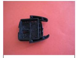
5. Old buttons are an over mould to the cover and have to be removed
